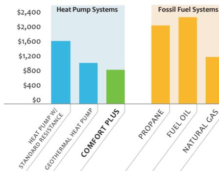
a day. During on-peak hours or when the demand for heat is at the point where the heat pump's capacity alone cannot satisfy the heating requirements, the Comfort Plus unit uses its stored, off-peak heat to supplement the heat pump output.
